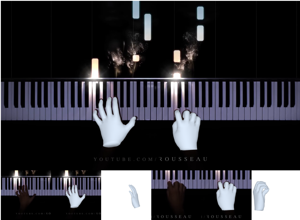
Figure 5: Hand reconstruction examples on Twinkle Twinkle Rousseau. On the top, we visualize the image-aligned 3D hand meshes from a birds-eye view, overlaid on the original video frame. On the bottom, we visualize the left and right hand meshes from a side view. Although the hand meshes are aligned with the input view, the depth of the fingers is inaccurate. For the left hand, only the little finger is actually depressed, even though both the little finger and middle finger are depressed in the hand mesh. For the right hand, only the index finger is actually depressed, even though the thumb is the only depressed finger in the hand mesh.
