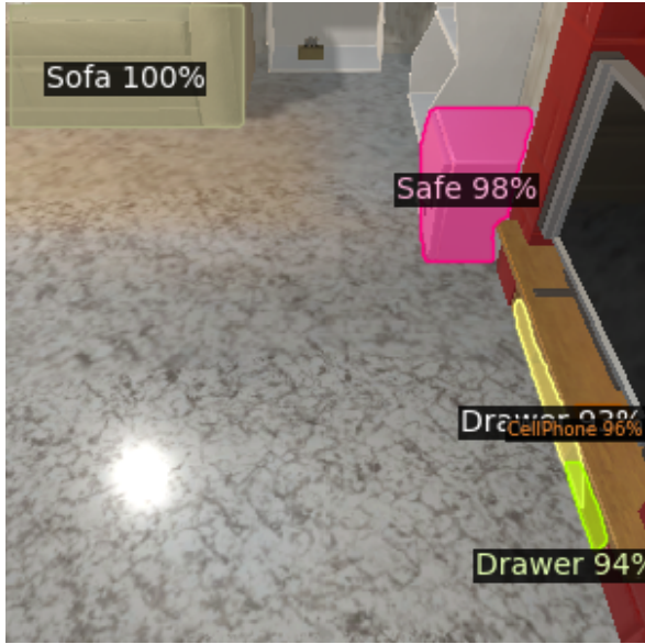
Figure 8: A part of the TV drawer is wrongly detected as the CellPhone object in the task.
